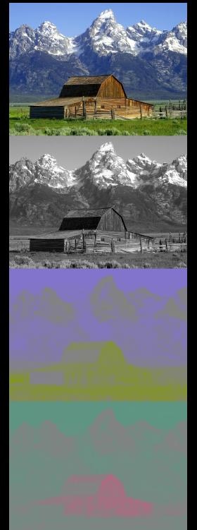
$Y'PbPr$  is then encoded to 8 bits per component
